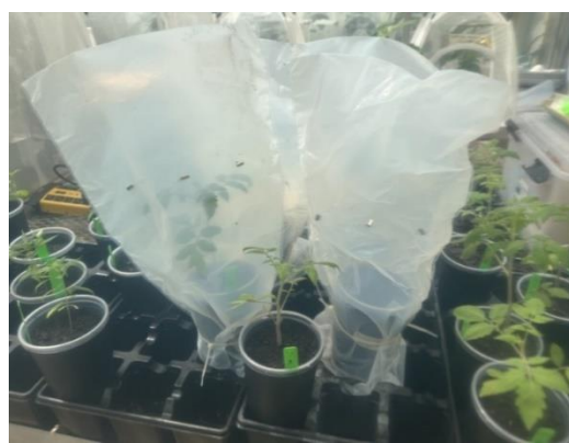
Figure 2: Close up of VOC collection. Tomato plants are placed into branch enclosures (Teflon bags). The material allows for photosynthetically active radiation to pass through, and tubing provides fresh air. Twisters are suspended to the sides of the bags, slightly above the plants, through magnets
