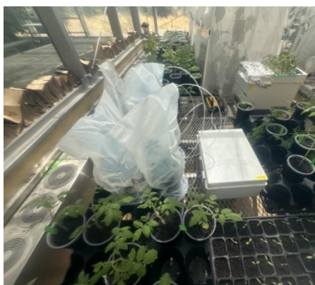
Figure 1: With limited space in the CRF, we created a flow manifold that allows simultaneous VOC collection from four plants.
