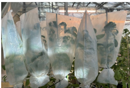
Figure 3: Close up of VOC collection. Tomato plants are placed into branch enclosures (Teflon bags). The material allows for photosynthetically active radiation to pass through, and tubing provides fresh air. Twisters are suspended to the sides of the bags, slightly above the plants, through magnet
